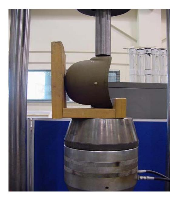
FIGURE 5. Jig for side to side compression resistance.
